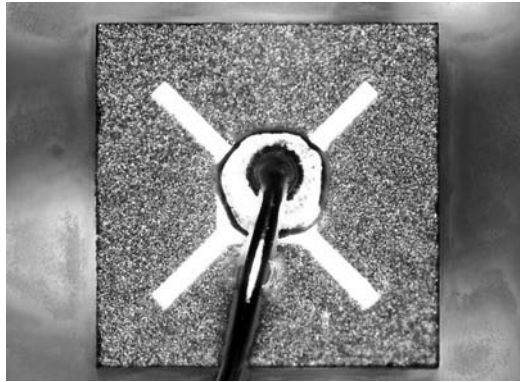
Figure 10.6 Photograph of a typical surface-emitting LED chip; the length of one side is 360\ \mu\text{m} . The X-shaped pattern is the surface electrical contact and the bond wire is seen emerging toward the bottom of the photo. Photograph courtesy of Robert Gehrke.
