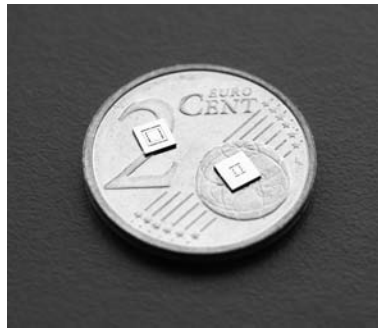
Figure 6.9 Silicon-based two-dimensional scanning micromirrors on a 2-cent coin, with two differing mirror sizes. The chip sizes for both are 3 \times 3 mm. Photo courtesy of Khaled Aljassem.
