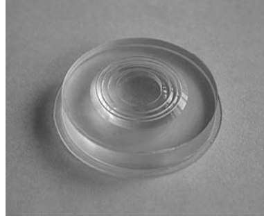
(b) Injection-molded discrete Fresnel lens, fabricated using the mold on the left; diameter of the inner lens structure (the Fresnel zones) is 25 mm.
